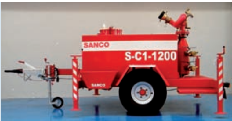
Top: wheeled drive, stainless steel welded monitor installed on the top of a vehicle Below: tank-mounted trailer monitor.
