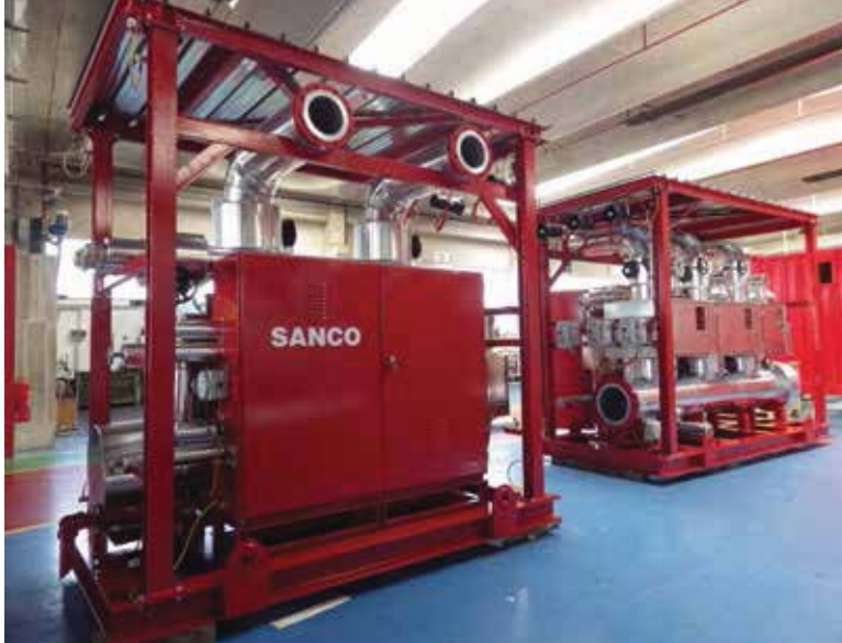
Fig. 6 - Uzbekistan project: deluge valves for very low temperatures
