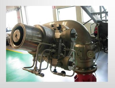
A mobile version (model RED TYPHOON) has been designed for high-risk operations (hydrocarbon tanks, chemical / petrochemical complexes and oil refineries, conventional and nuclear power plants).
